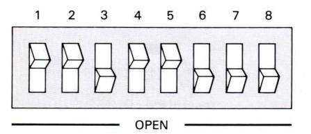
**Figure 12.** Recommended dip switch setting for connecting the Houston Instruments Model DMP-29 Plotter to your computer
