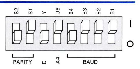
**Figure 11.** Recommended dip switch setting for connecting the Hewlett-Packard Model 7470A Plotter to your computer
