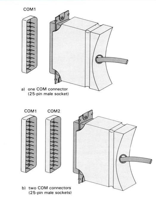
Figure 7. Two COM connector setups
