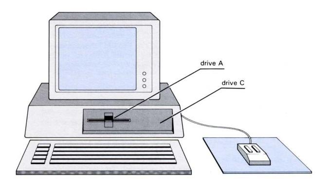
**Figure 4.** The IBM Personal Computer XT has the one floppy disk drive set up as drive A and the hard disk drive as drive C.
