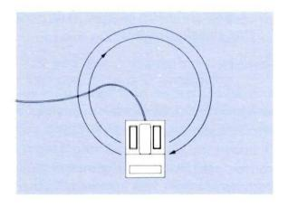
**Figure 8.** To calibrate the mouse, slowly move it in 9-inch circles on the pad twice. If the mouse doesn't calibrate, move it in large circles again.
