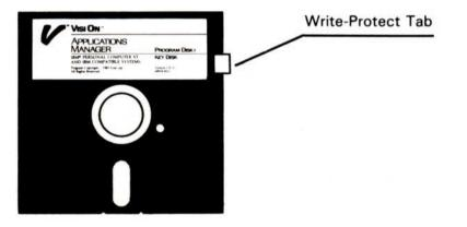
**Figure 5a.** The write-protect tab on the Visi On Program Disk 1 (Key Disk) protects the information on the disk.
