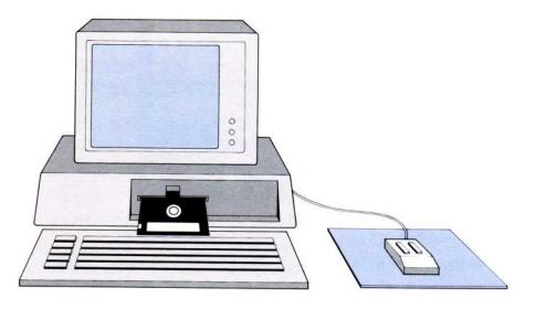
**Figure 6.** Carefully insert the disk into the drive with the label entering last.
